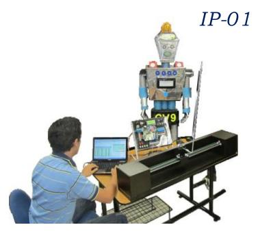
The inverted pendulum is an excellent lab practice for those interested in control, systems, mechanics, process, electronics, mechatronics and robotics. This is a very fundamental application for robotics to understand among other concepts, the equilibrium concept.
